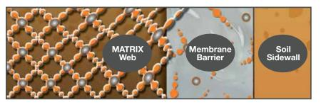
The BIG-FOOT<sup>®</sup> Polymer Slurry system works by creating a polymeric differential pressure barrier throughout the sidewall of the excavation. The polymer slurry reacts when it comes in contact with freshly exposed soil, creating an organized web of polymer strands. This web allows BIG-FOOT to bond to the sidewall of the excavation.
