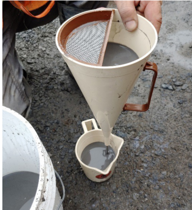
Measuring drilling fluid viscosity
