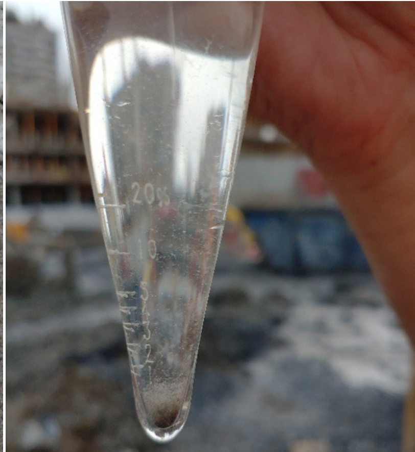
Checking sand content of drilling slurry
